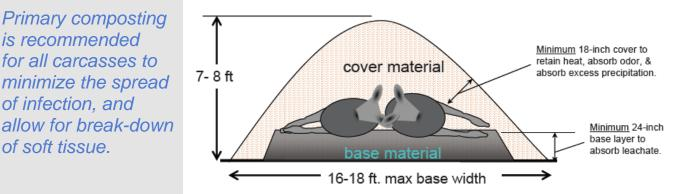
Figure 2. Placement for large carcasses (cattle and horses) in static pile composting.
