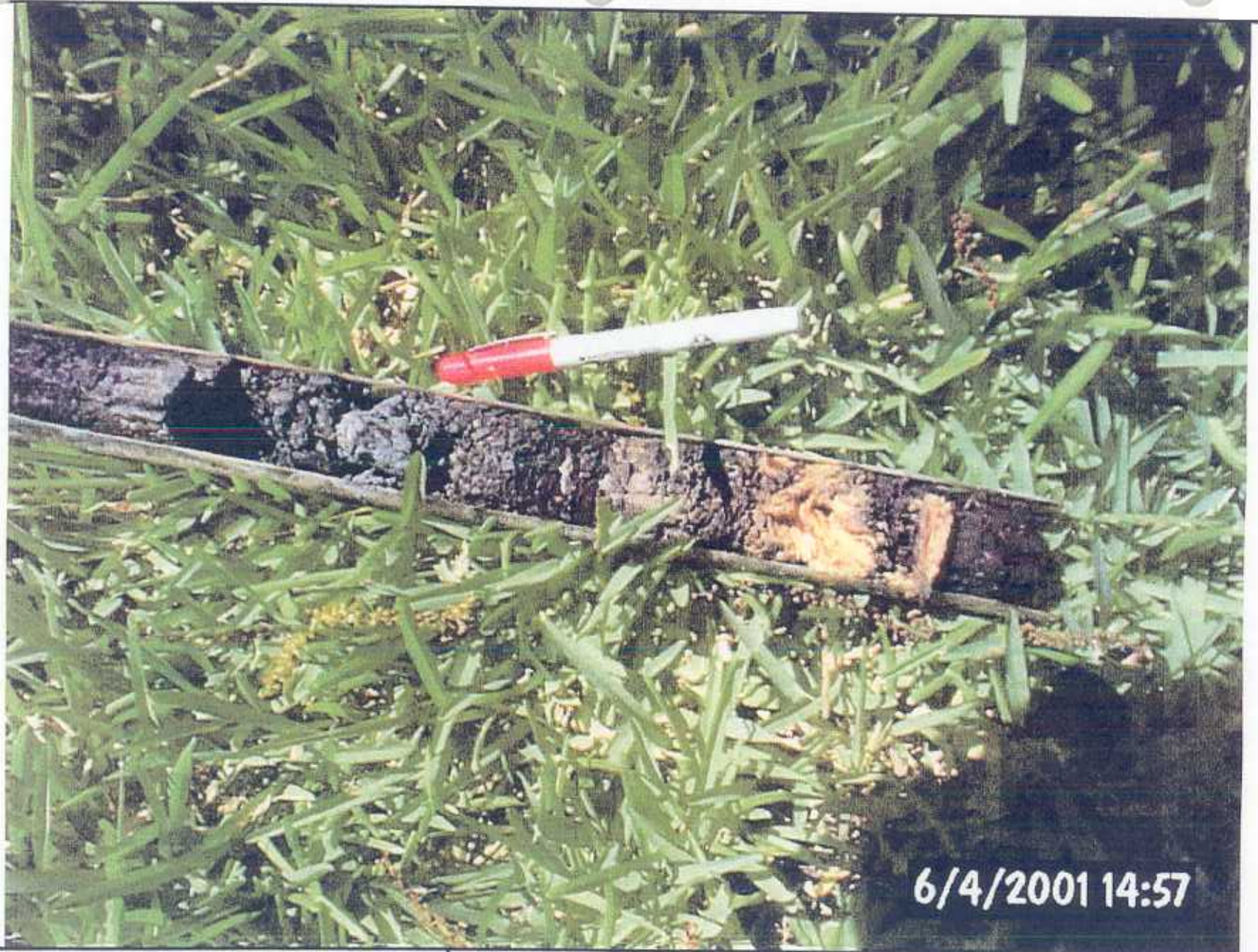
Photograph 7: Ash/Slag in SIS Core Sample Mill View Subdivision Study Site Port St. Joe, Gulf County, Florida
