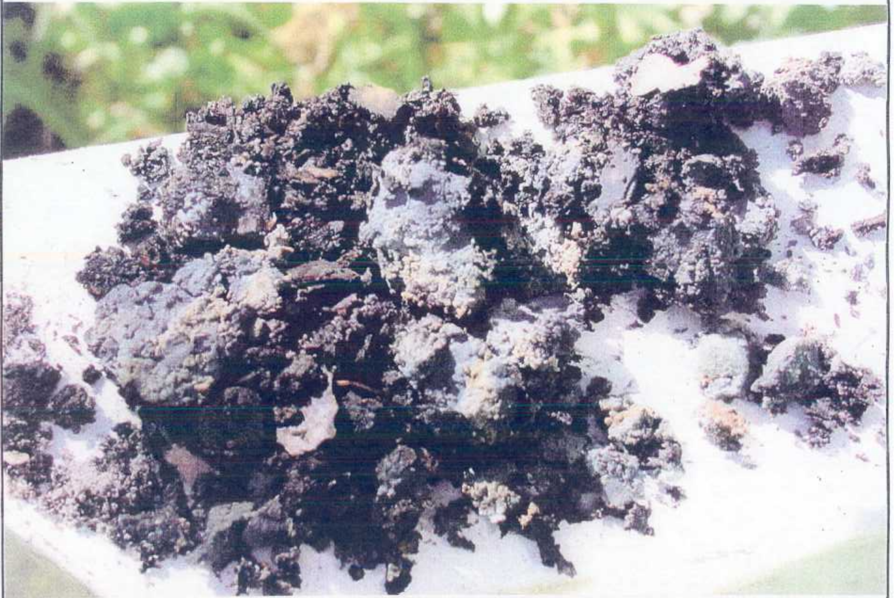
Photograph 8: Lime Grits in Blue/Green Clayey Matrix Mill View Subdivision Study Site Port St. Joe, Gulf County, Florida
