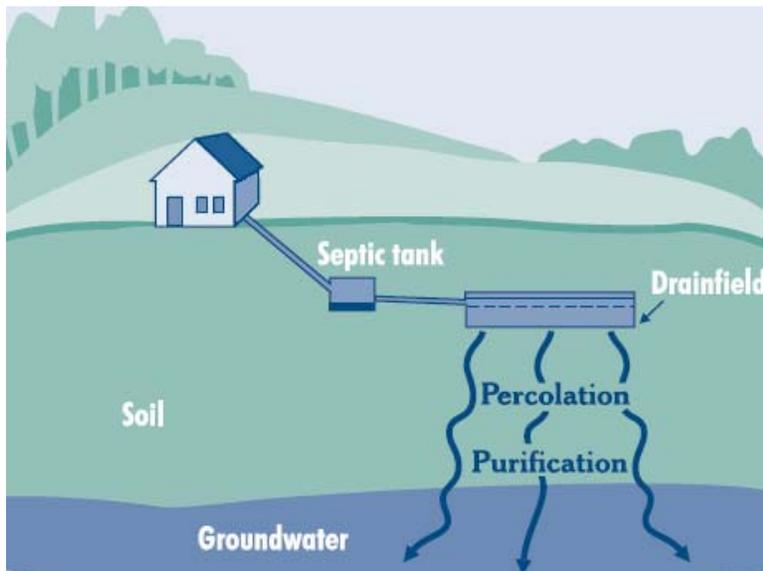
Figure1-1. Conventional onsite sewage treatment and disposal system (septic system) (from [http://www.epa.gov/owm/septic/pubs/homeowner\\_guide\\_long.pdf](http://www.epa.gov/owm/septic/pubs/homeowner_guide_long.pdf)).
