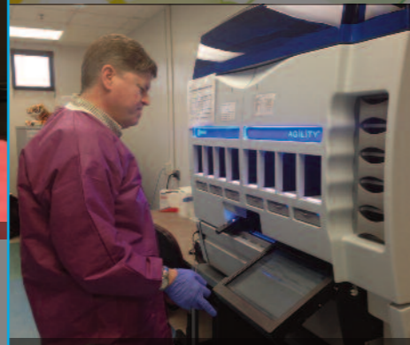
All RPR positive specimens are reflexed to Trinity BioTech's TrepSure EIA (total antibody IgG + IgM) assay using Dynex Agility automated EIA processor. This instrument performs all the specimen and reagent handling and pipetting, washing, incubation, absorbance detection and calculation of results. The EIA instrument provides for positive identification of specimens and automatic download of results when interfaced with Labware.
