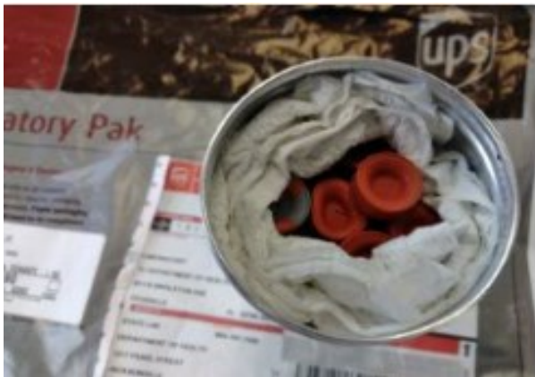
Secondary container over-filled. Improper cushioning of primaries could result in leaks.
