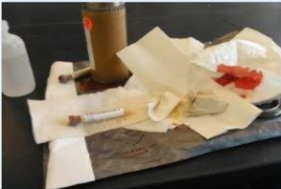
Improper packaging results in broken primaries causing potential risk of exposure and sharps hazard.
