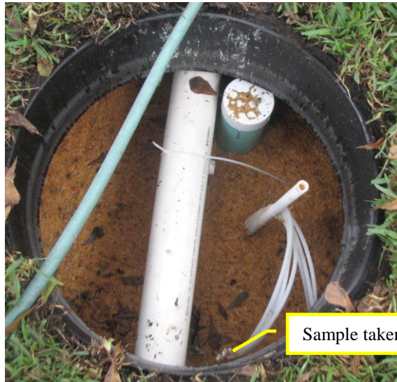
Figure 7 First chamber of Stage 2 biofilter (B-HS2-LIGNO-0" sample)
