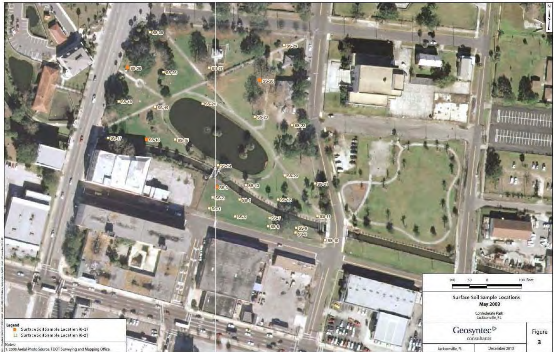
Figure 3. Main Street MGP/Confederate Park Site Surface Soil Sample Locations
