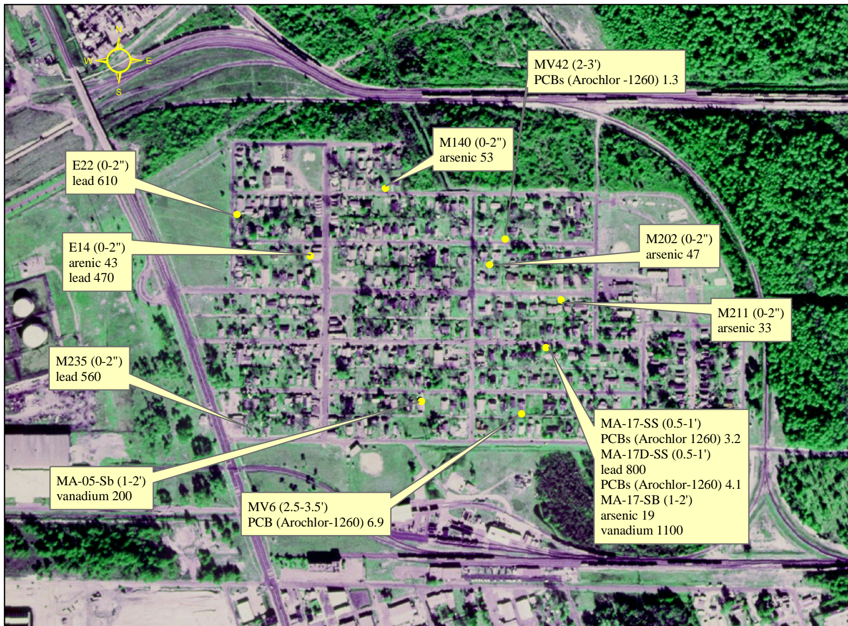
Figure 3: Chemicals measured in soil (in mg/kg) that exceeded Minimum Risk Levels, and lead above the DEP Soil Target Cleanup Levels. MA data are from EPA 2002, MV data are from DEP 2002, M and E data are from Flowers.
