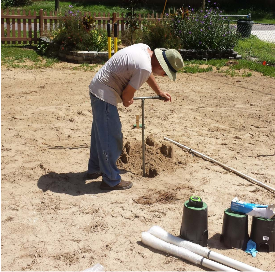
Lysimeters installed in hand augered boreholes
