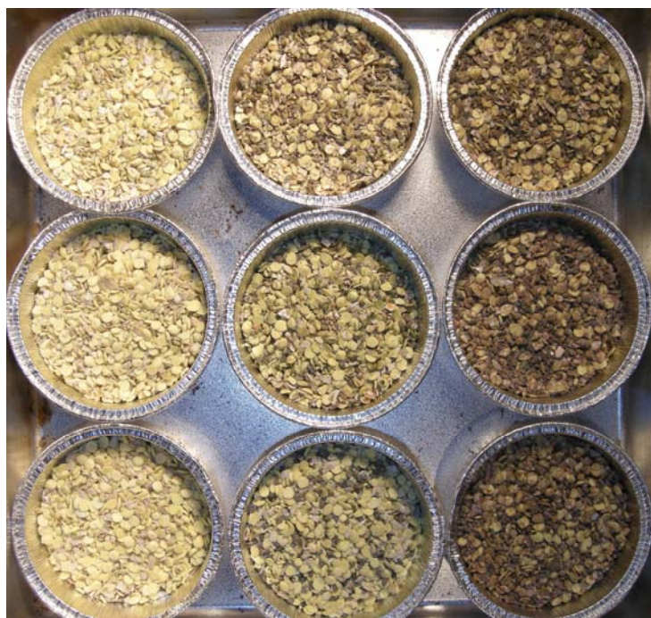
Figure 21 Stage 2 Media Dried at 103C (Day 246). Left to right, Column 2A, 2B, 2C. Top to bottom in direction of column entrance to exit.
