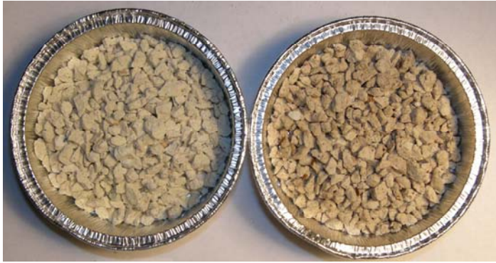
Figure 17 Clinoptilolite: New (left) and Column 1A Upper Layer Dried at 103C (Day 246)
