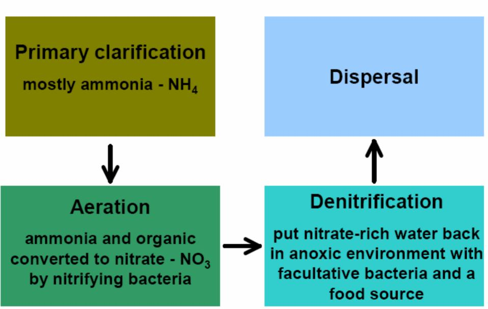
Schematic of Typical Onsite Wastewater Nutrient Reduction System (OWNRS) for the Florida Keys
