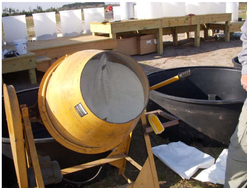
Mixing Media (Clinoptilolite 8X14 and Oyster Shell)
