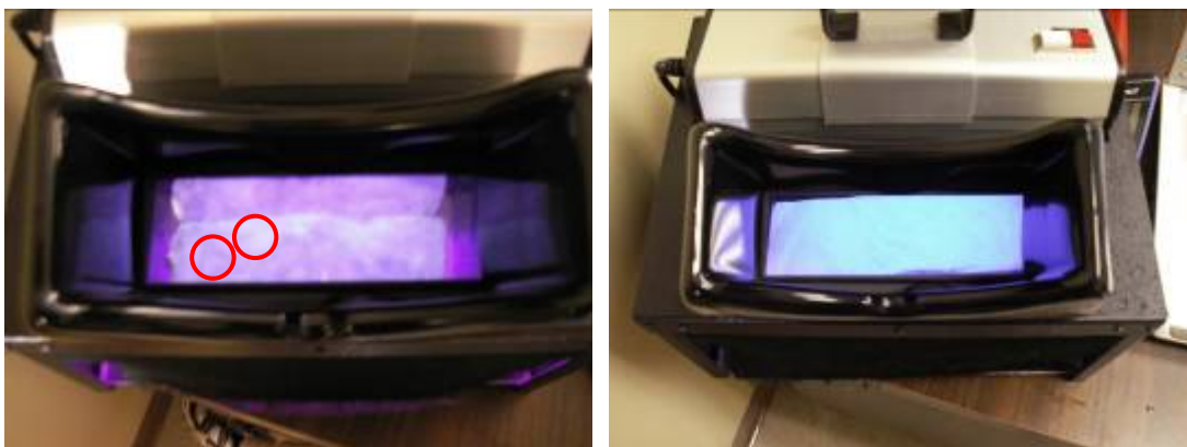
Figure 35 - A field collected optical brightener pad (Dekle Beach collected on 12/14/2006). In the left picture, a clean pad is shown on top to compare with the collected pad on the bottom. Very tiny flakes are visible under ultraviolet illumination (circled). In the right picture, a pad with optical brighteners is shown for comparison. Notice the same blue fluorescence seen for the tiny flakes on the left.
