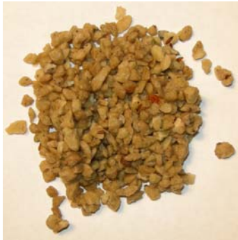
Figure 14 Clinoptilolite Media from Upper Layer (Day 246).
