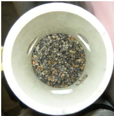
Figure 12 Surface of Expanded Clay Filter (Day 246).
