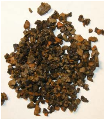
Figure 15 Expanded Clay Media from Upper Layer (Day 246).
