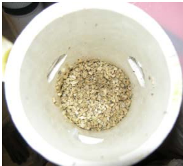
Figure 11 Surface of Clinoptilolite Filter (Day 246).
