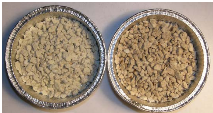
Figure 17 Clinoptilolite: New and Column 1A Upper Layer Dried at 103C (Day 246) (Left: new)
