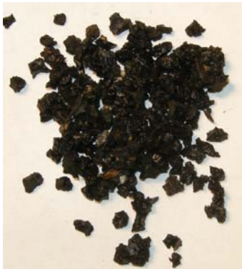
Figure 16 Granular Rubber Media from Upper Layer (Day 246).
