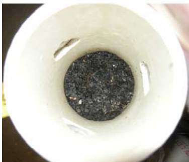
Figure 13 Surface of Granular Rubber Filter (Day 246).
