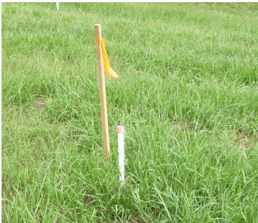
Figure 3 Installed 3/4" Diameter PVC Standpipe Piezometer
