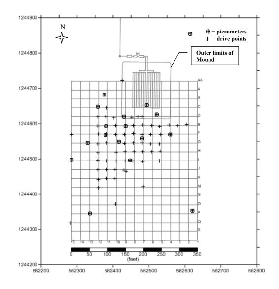
Figure 1 Schematic of GCREC Monitoring Network (UTM coordinates are used) **⊕** denotes piezometers and + denotes drive points
