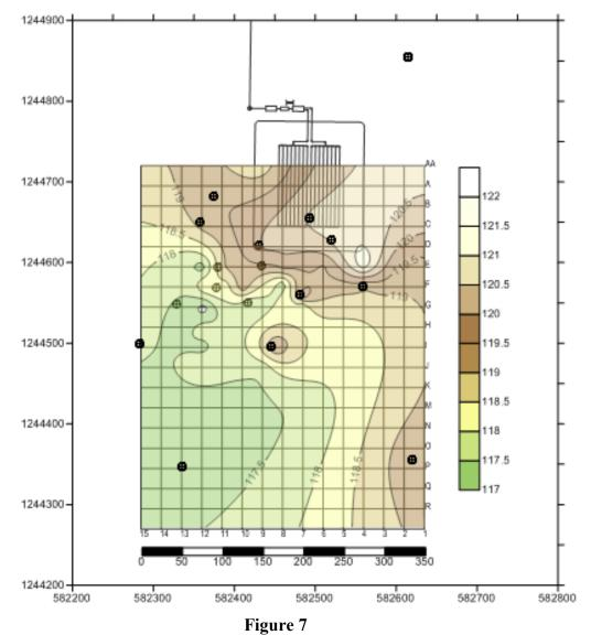
Elevations of Spodic Layer as Determined by Hand Held Methods (The locations of the piezometers are provided for reference.)
