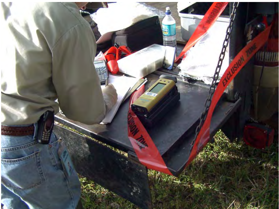
Photo 6: January/February 2003, L-level x-ray fluorescence instrument used in soil screening.
