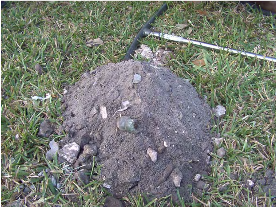
Photo 3: January\February 2003, surface soil boring containing debris.
