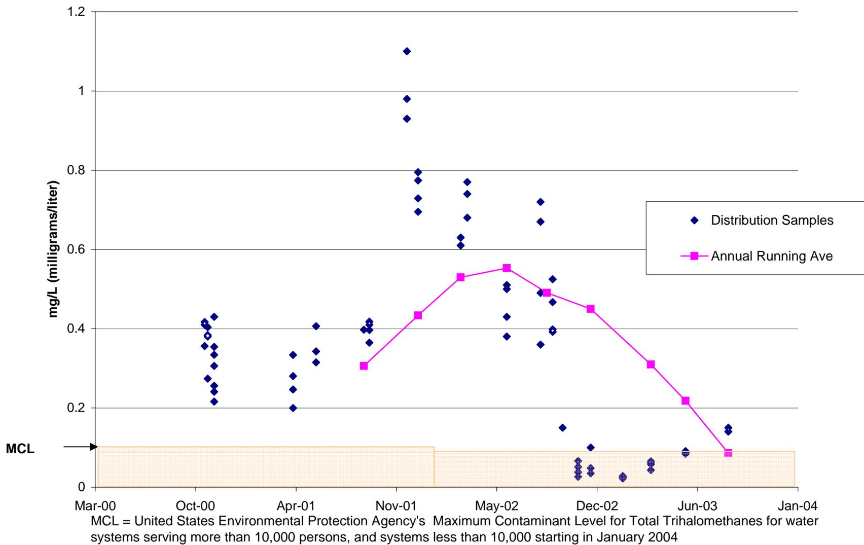
**Figure 4 - Total Trihalomethane Levels (THM) Levels in South Bay, Florida Municipal Water System - Distribution Samples**
