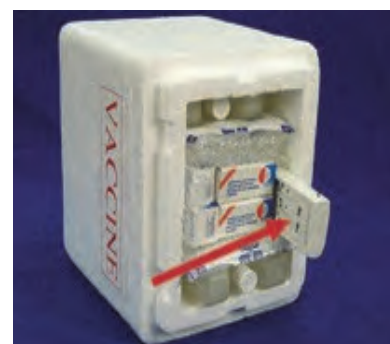
Place a thermometer next to the vaccine but not in contact with the refrigerated/frozen packs.
