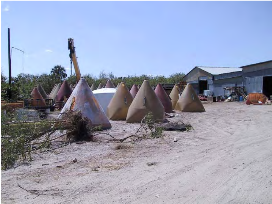
Photo 3. Fiberglass forms at Tampa Fiberglass.
