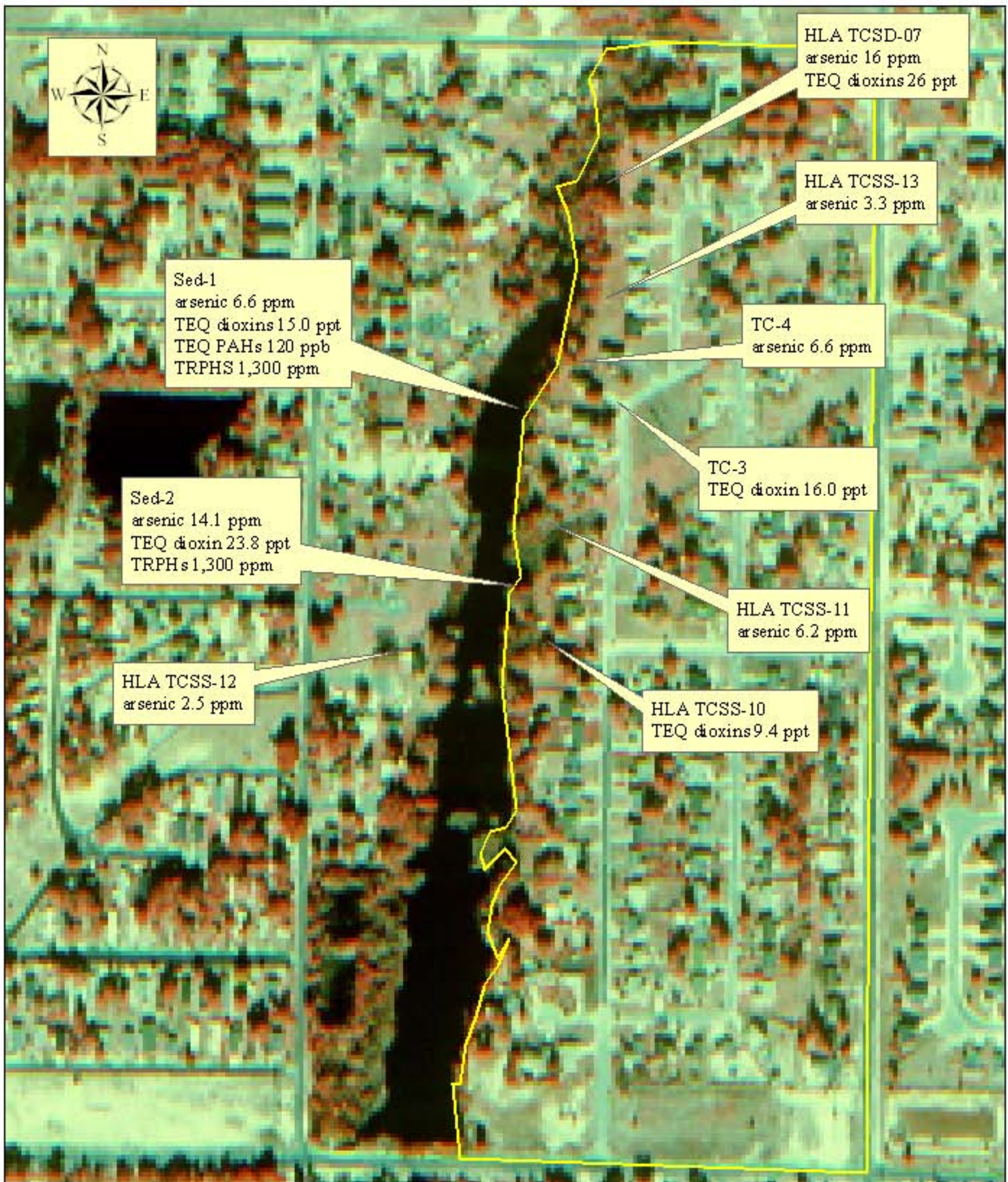
Figure 3: Approximate locations of soil or sediment samples with chemicals measured above residential Soil Cleanup Target Levels in and near the Town and Country Lake Estates
