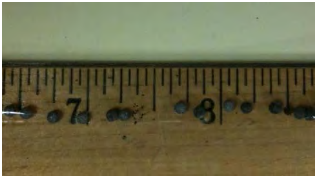
Figure 11. Lead shot taken from playground during site visit and placed on ruler for size comparison. Photos Taken by Julie Corkran EPA June 2009. Measurement of lead shot.
