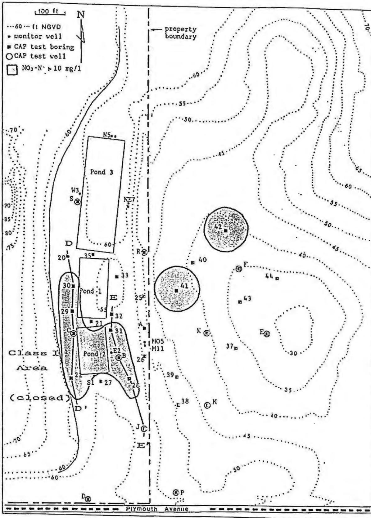
Figure 4. --Soil Boring and Monitor Well Locations.
