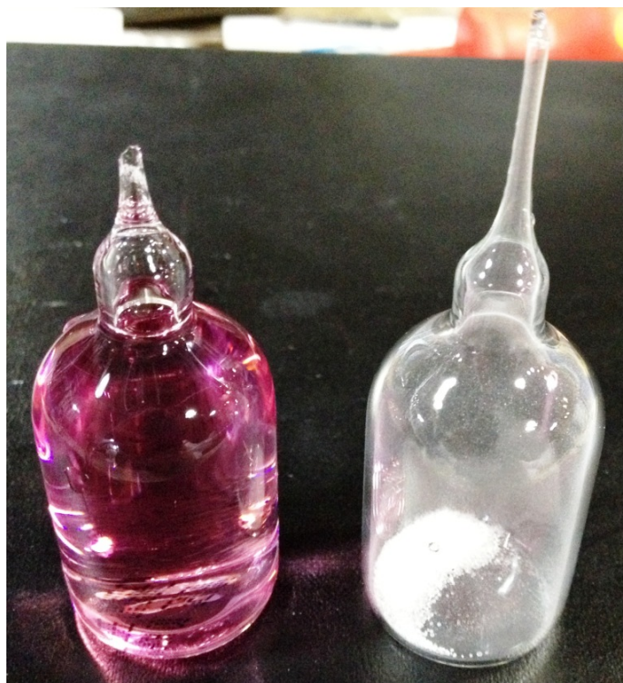
Figure 2 - Hach DPD AccuVac (Used & Unused)
