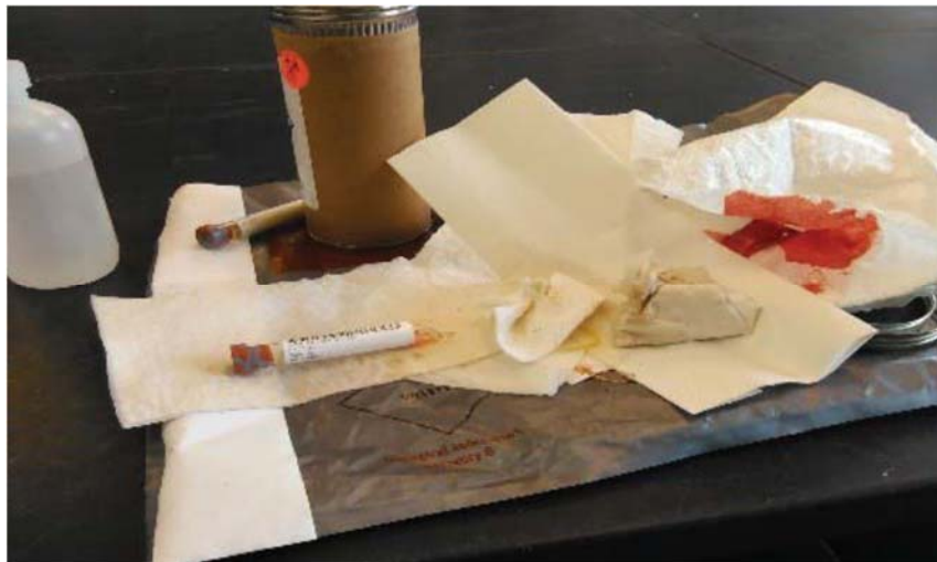
Insufficient cushioning resulting in broken primaries.
