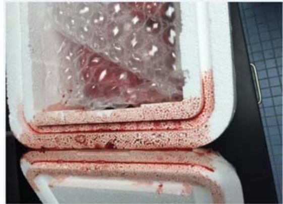
Example of a shipment that lacked sufficient amount of absorbent material, and the primary and secondary packagings were not leak proof.
