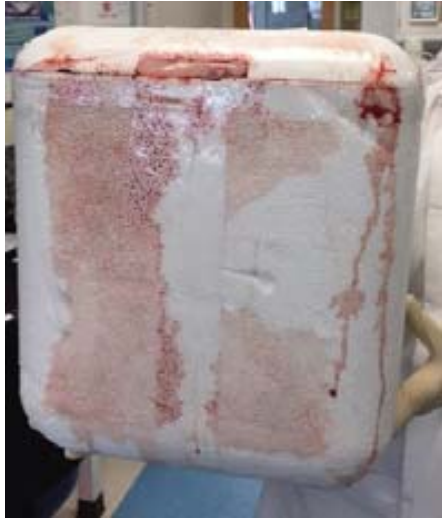
Example of a shipment that lacked sufficient amount of absorbent material, and the primary and secondary packagings were not leak proof.
