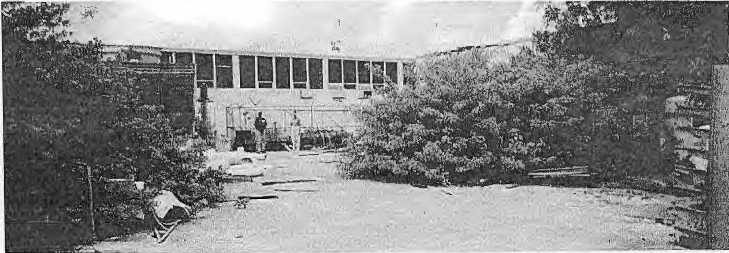
**Photo 4: Southwest corner of the northern building. Window above Donald Sikaswe's head is broken, revealing asbestos insulation around piping. Rusty metal equipment could be a physical hazard.**
