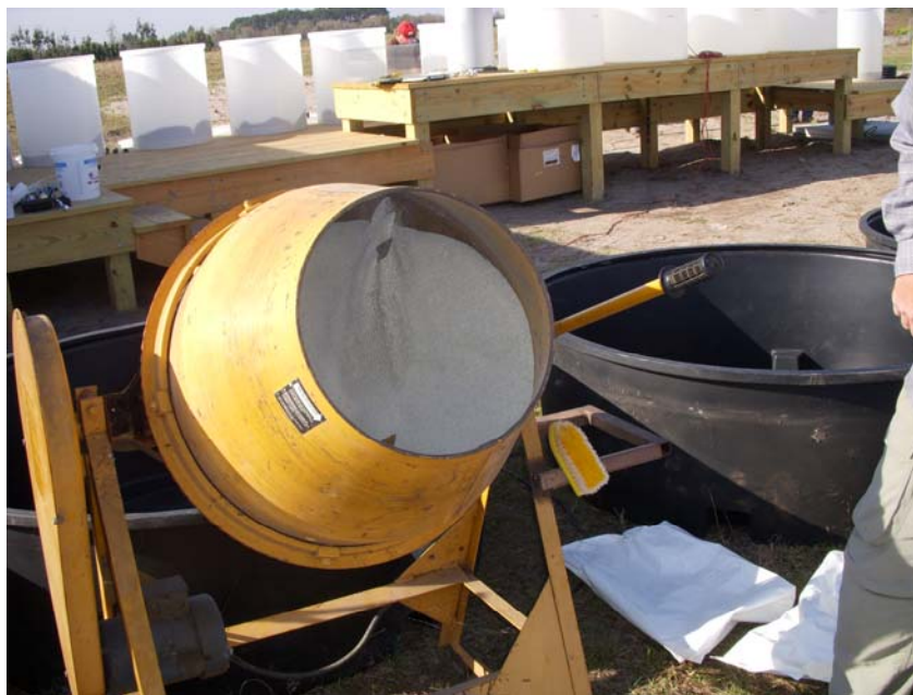
Mixing Media (Clinoptilolite 8X14 and Oyster Shell)
