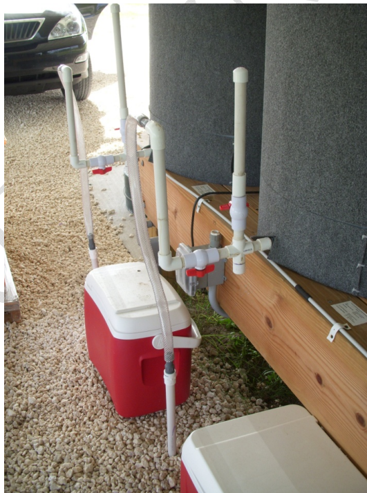
Figure A.2 Revised In-situ Simulators Discharge Piping 7/20/10
