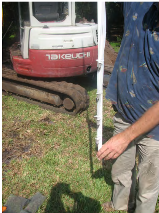
Figure 24 Stage 2 biofilter tank SST drivepoint sampler tree (sulfur chamber)
