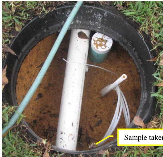
Figure 7 First chamber of Stage 2 biofilter (B-HS2-LIGNO-0" sample)
