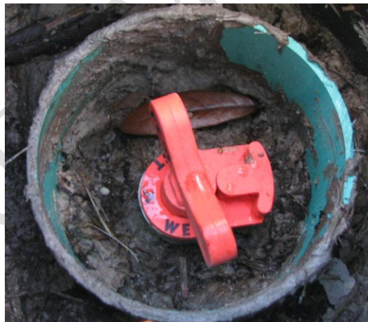
Figure 8 Treated Effluent Suction Lysimeter (B-HS3-LY03 and –LY04 sample)
