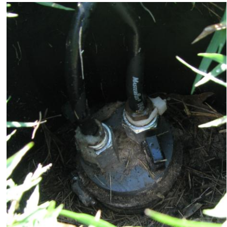
Figure 6 Stage 1 Suction Lysimeter (B-HS3-LY01 and -LY02 sample)
