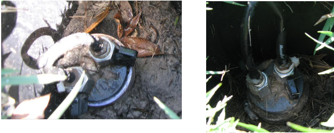
Figure 5 Stage 1 Suction Lysimeter (BHS3-LY01 and –LY02)
