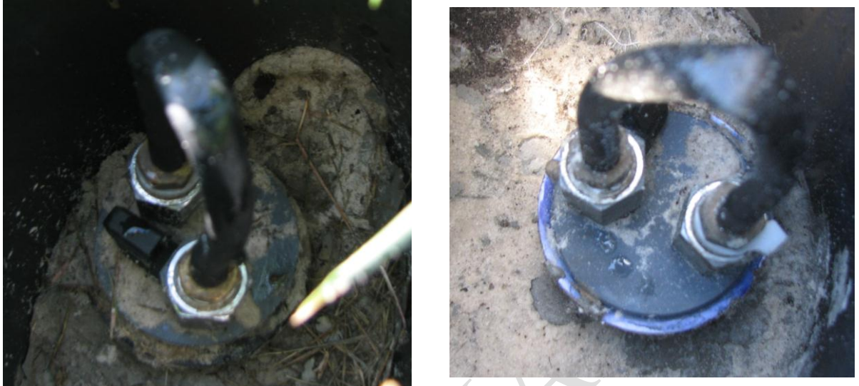
Figure 7 Treated Effluent Suction Lysimeter (B-HS3-LY03 and -LY04 sample)
