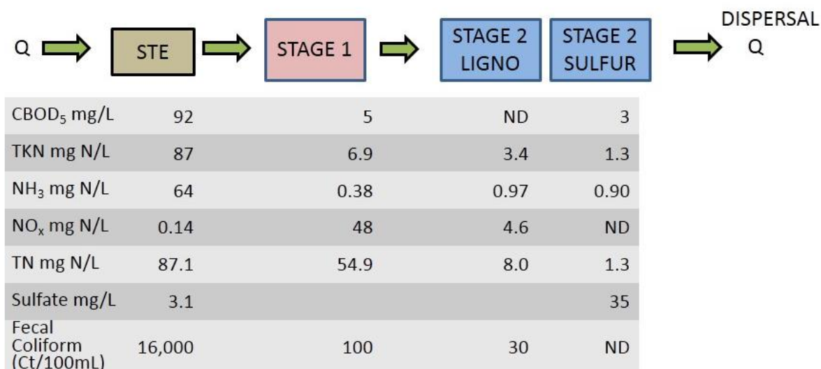
Figure 8 Graphical Representation of Nitrogen Results Sample Event No. 1 September 30, 2013 (Experimental Day 83)
