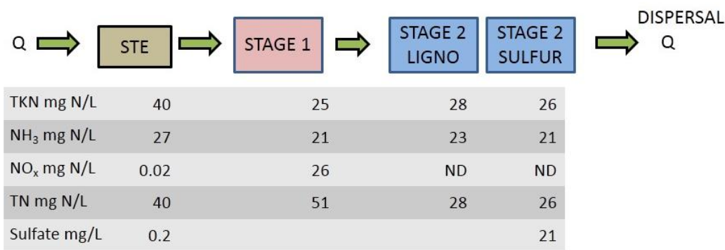
Figure 7 Graphical Representation of Nitrogen Results Preliminary Sample Event July 29, 2013 (Experimental Day 20)
