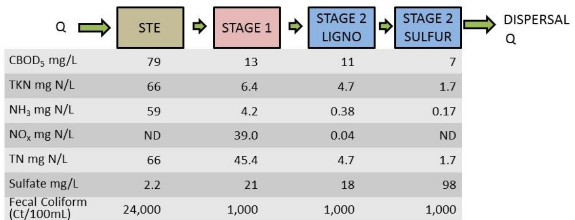
Figure 8 Graphical Representation of Nitrogen Results Sample Event No. 3, February 3, 2014 (Experimental Day 209)
