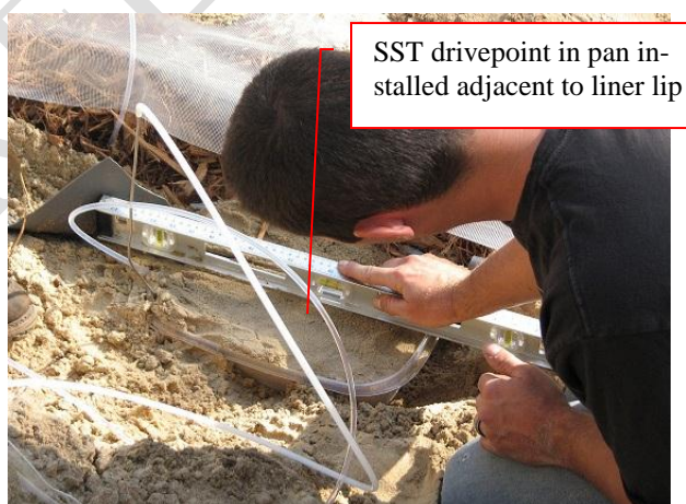
Figure 11 Treated effluent sample taken from drivepoint in pan (BHS7-EFF-DP samples)
