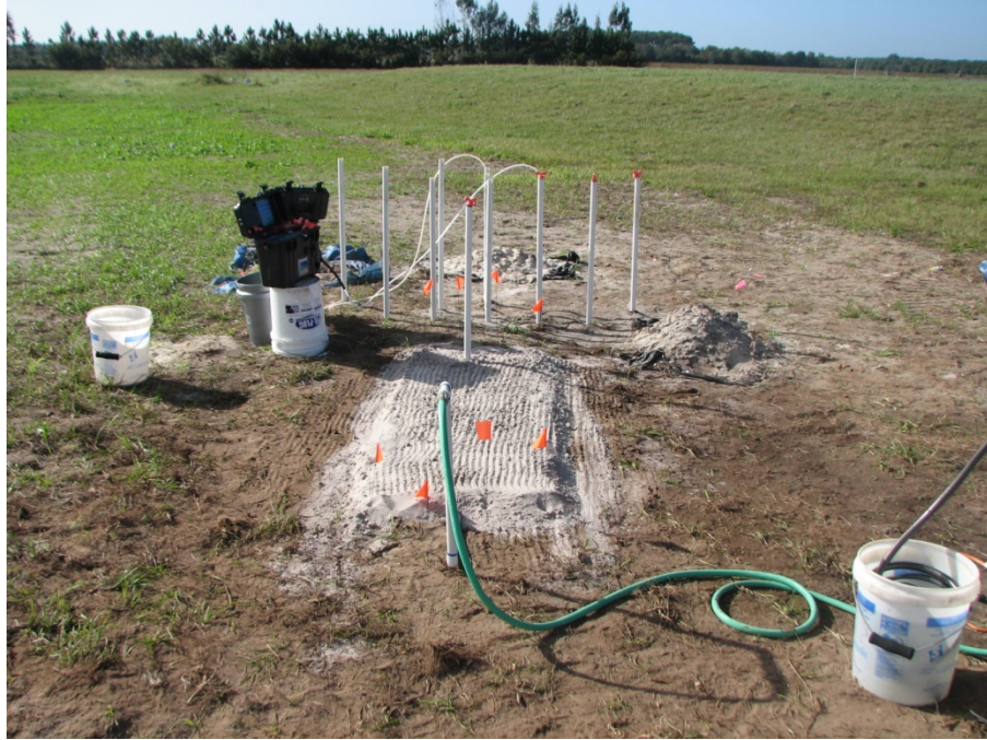
Figure 3 Tracer test area with initial wells installed downgradient
