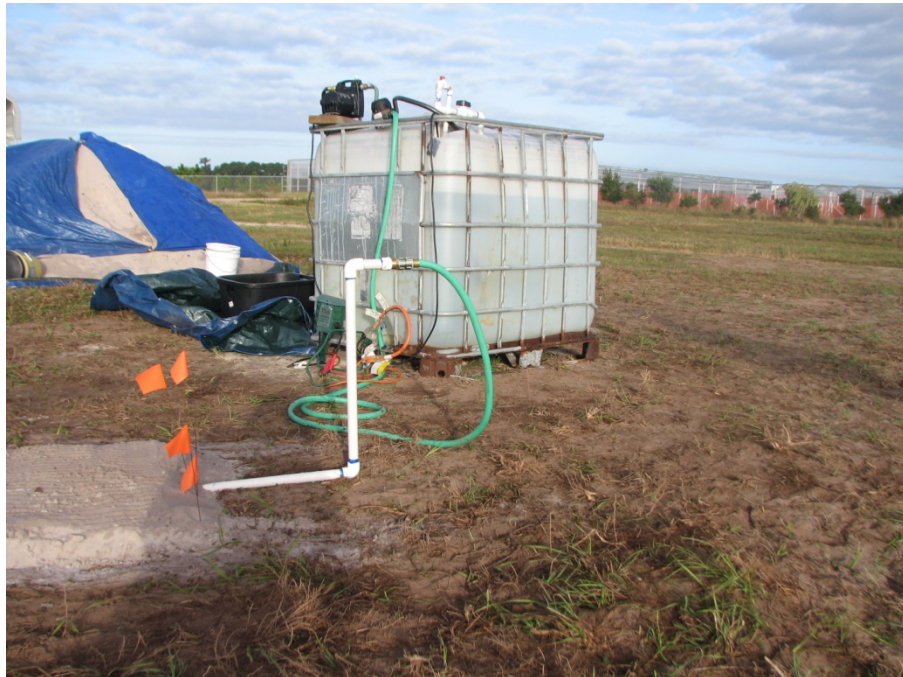
Figure 4 The 250-gallon tank containing the tracer solution, dosing pump on top of tank
