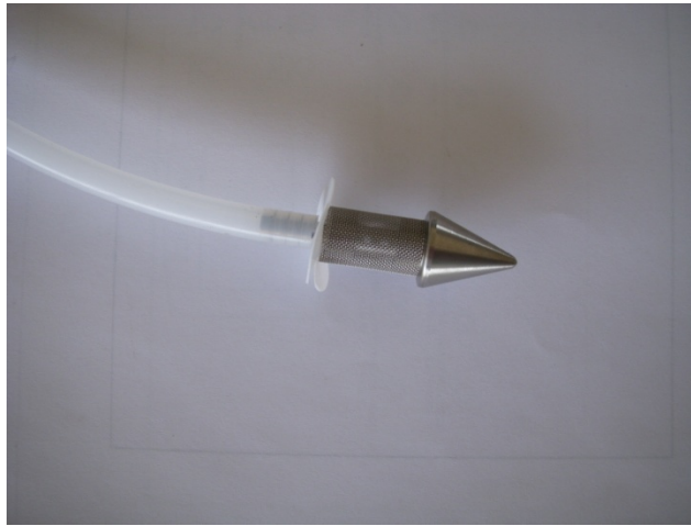
Figure 2 Stainless Steel Drive Point with Mesh Screen, Umbrella and Tubing
