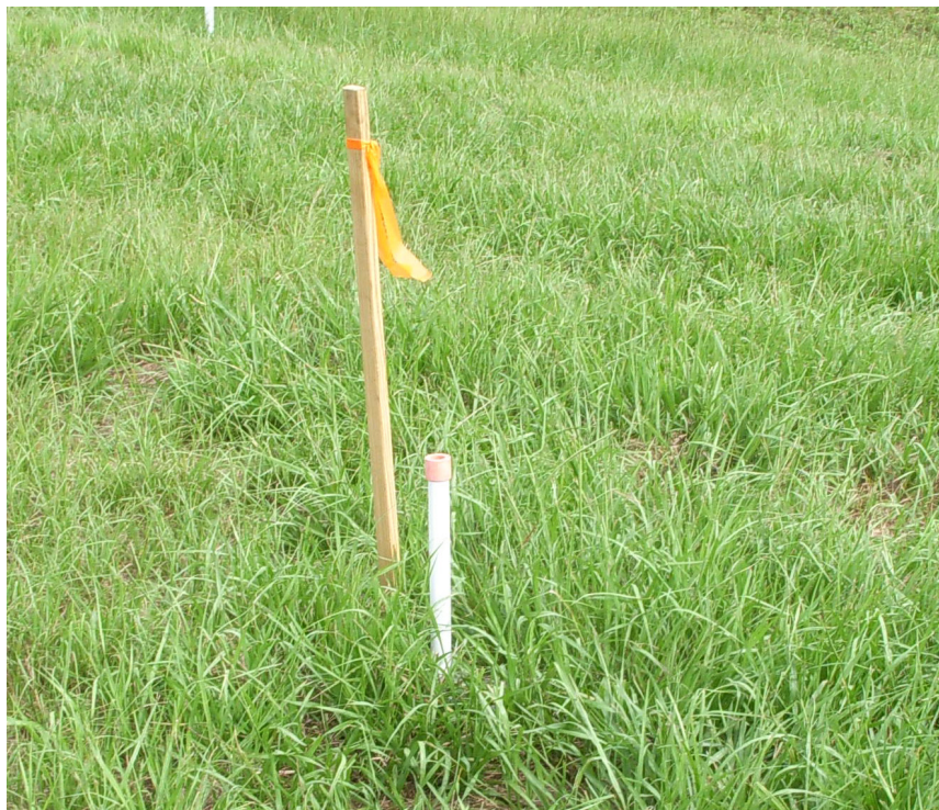
Figure 3 Installed 3/4" Diameter PVC Standpipe Piezometer
