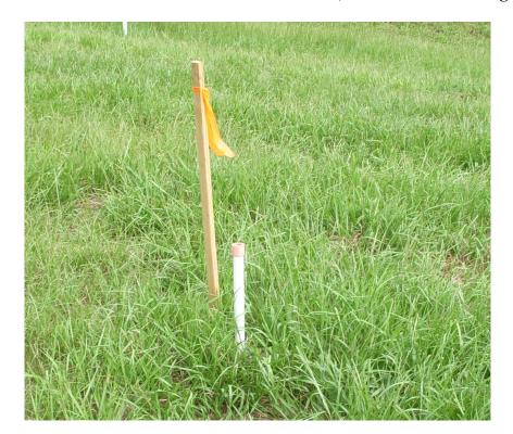
Figure 3 Installed <sup>3</sup>/<sub>4</sub>" Diameter PVC Standpipe Piezometer
