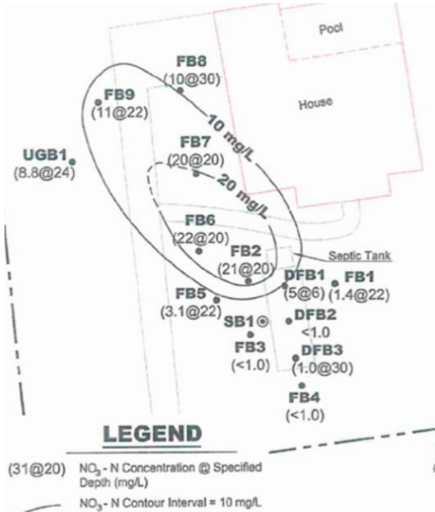
Figure 2-3: Plume Illustration Showing a Plot of Measured Concentrations for Aerial Views of a Nitrate Plume in Lake County, Florida
