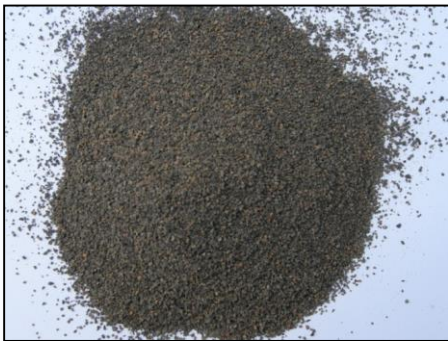
nitrification media: expanded clay
