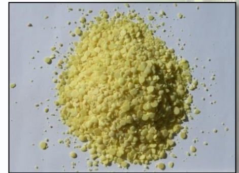
denitrification media: elemental sulfur
